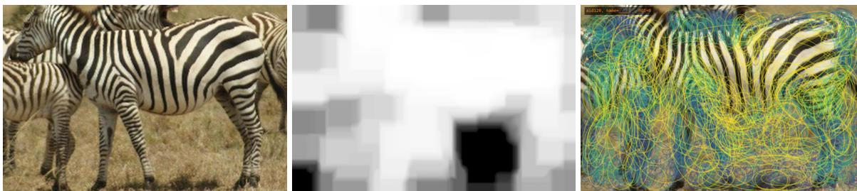
**Figure 3.15: The locations of SIFT keypoints are not semantically constrained to the animal body and, if added to an identification search database, can confuse the ranking algorithm and exacerbate known issues like scenery matching. The coarse background segmentation model allows for SIFT keypoints to be down-weighted based on how much they contain background information. Yellow keypoints have a higher weight compared to blue keypoints.**
